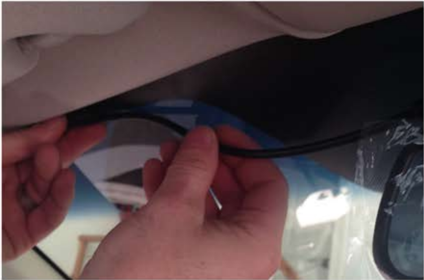
Tuck wire from SmartNav 5 into headliner. It only has to go in just a little to stay in place.
