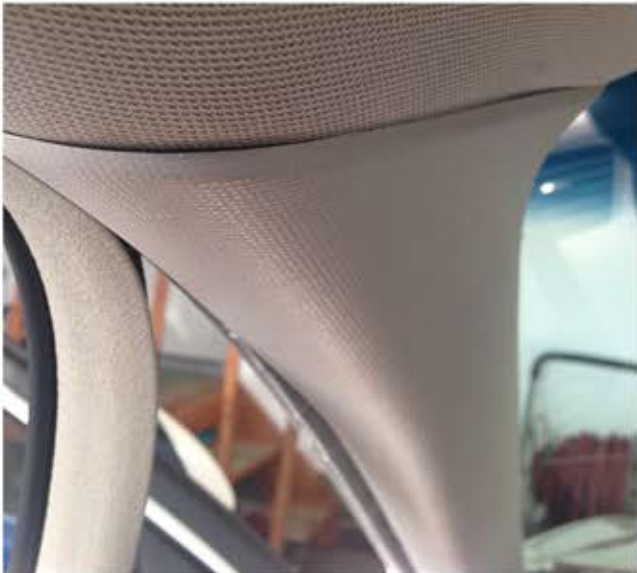
Route to which ever pillar A or B will get you to your power source. In this case it was A pillar, the Driver side.
