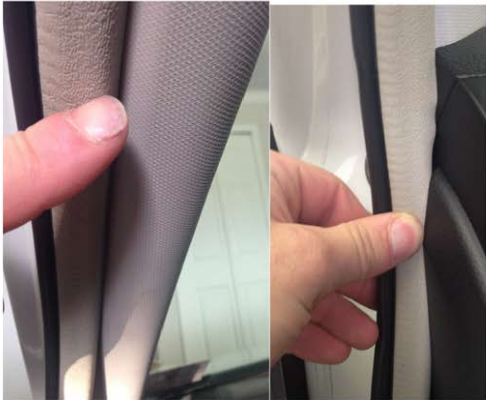
Remove weather stripping and run wire harness behind it. As you come down the pillar, tuck weather stripping back into place pressing firmly. You may need to use a plastic wedge tool to force back behind dash.
